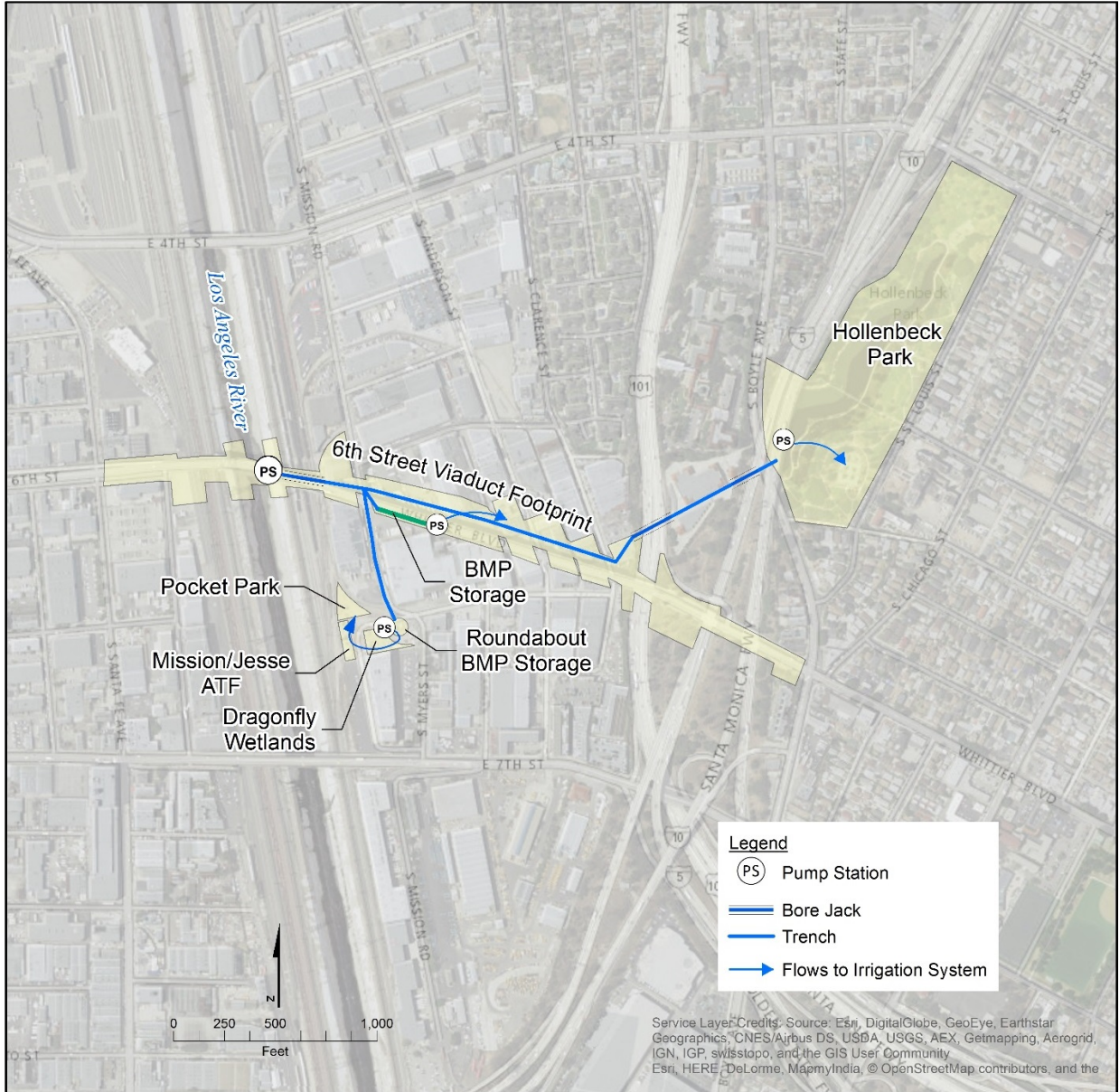
Figure 3-3. Conceptual Conveyance Alignment, Water Supply Alternative: Los Angeles River Hollenbeck Park Lake Rehabilitation and Stormwater Management
